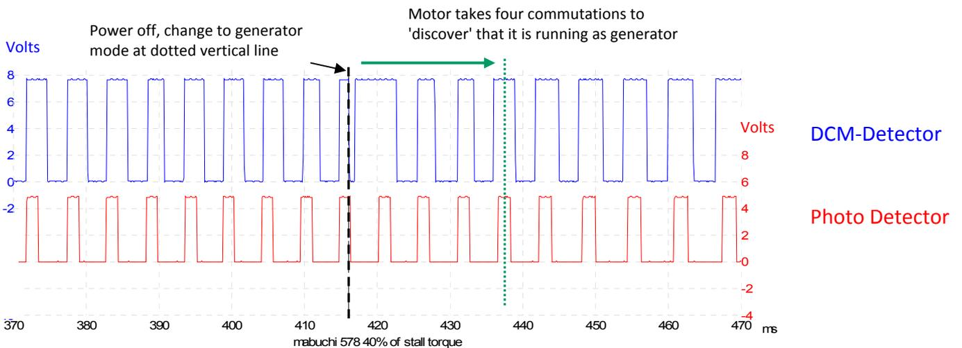
Fig. 2. Details of counts when changing from motor mode to generator mode
