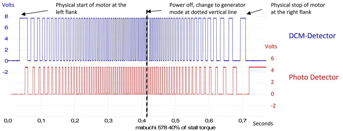
Fig. 1. DCM-Detector counts compared with photo detector counts at 40% of stall torque on a Mabuchi 578 8 pole motor.
